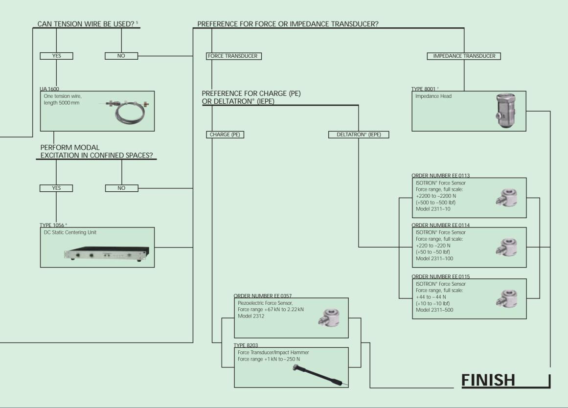
7. An impedance head provides for highest accuracy of the driving point frequency response function measurement as there is a perfect co-linear relationship between force and acceleration measurement. Note that use of the impedance head requires that the dynamic mass of the structure under test must be less than 1.5 kg for force measurement errors less than 10%. Structures with a dynamic weight of more than 1.5 kg should be instrumented with separate force transducers and accelerometers
